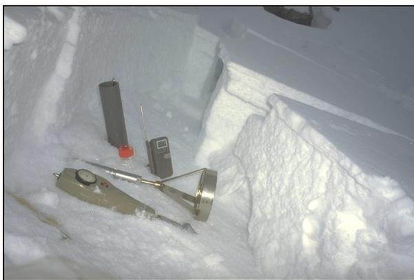
Figure 2. The snow layers are observed on the crown location : temperature, density, shear and ram resistance, and picking up of snow samples are performed.
