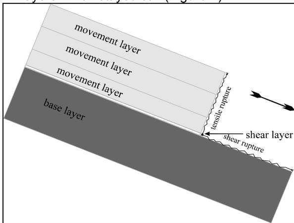
Figure 1. Three different layer types are taken into account on the crown.
