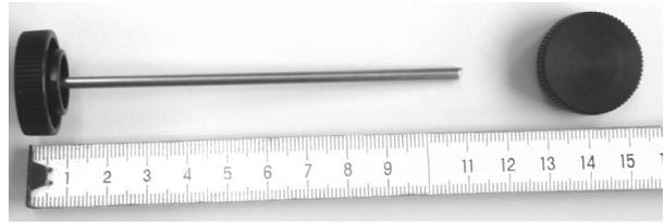
Figure 1: Black markers are used to visualize the deformation of the slab in the videos of the experiment. Shown here is an example of markers we use.
