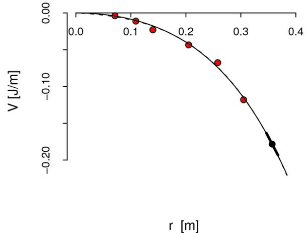
Figure 4: The mechanical energy ( $V$ ; red dots) was calculated for several cut lengths ( $r$ ). The slope of the fitted curve at the critical cut length (black dot with thick line) corresponds to the weak layer fracture energy.
