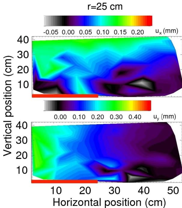
Figure 3: Displacement field for experiment A with a cut length of 25 cm. Upper panel: slope parallel displacement. Lower panel: slope normal displacement.
