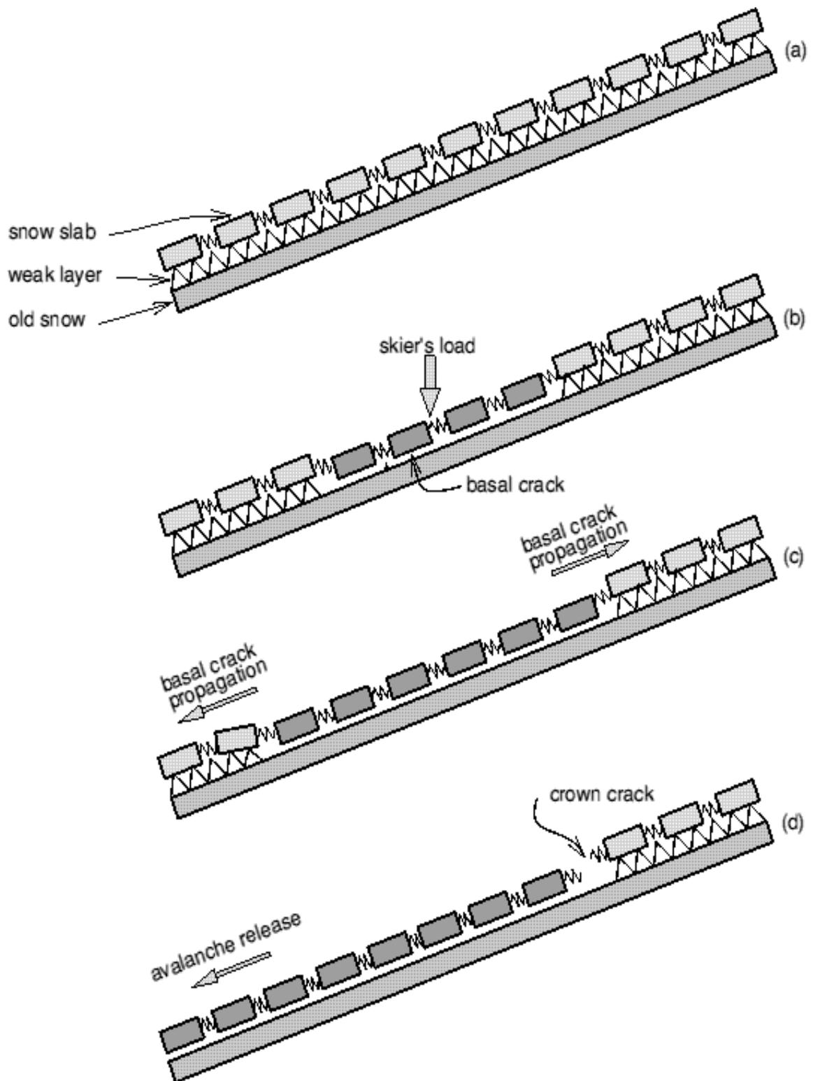
Figure 1. (a) A slab on a weak layer may be schematised as a series of blocks linked by elastic/brittle springs, lying on a collapsible house of cards; (b) the skier's load may collapse part of the house of cards (basal crack); (c) driven by either the skier's action or the snow weight, the basal crack may extend; (d) when the extension of the basal crack is large enough, the weight of the hung part of the slab initiates a crown crack at the top, resulting usually in the avalanche release.
